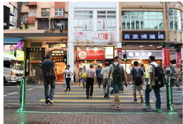
Figure 9. The Testing of the Prototype “Ground-level LED Light Strip” in the Healthy Street Lab
