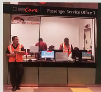
Height of service counter lowered with equipment to aid hearing impaired
